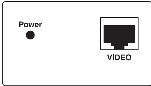
Figure 5. Remote unit rear view: Power LED, CAT5 port.
