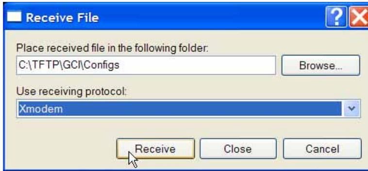
**Figure 6** – Make sure to select the Xmodem protocol and the proper directory where the configuration is saved. Click on Receive. This starts the file transfer.
