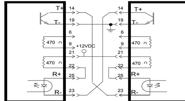
Figure 10. Interconnection of Two Current Loop Converters
