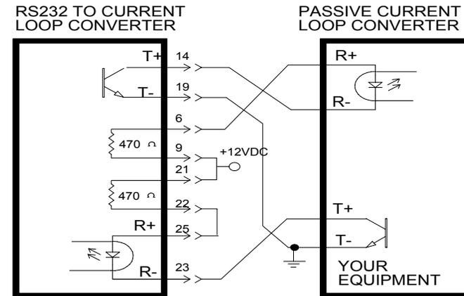
Figure 9. Connection to a Passive Current Loop
