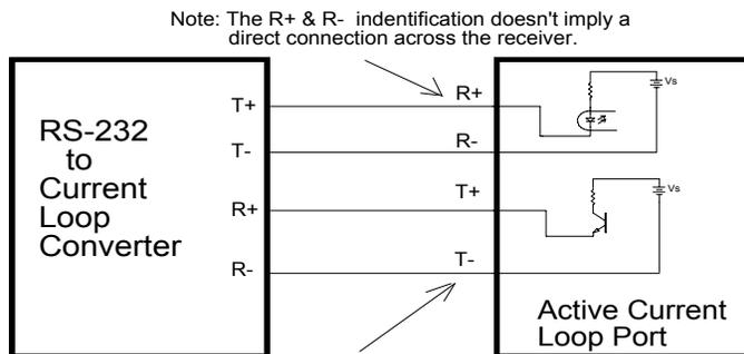
Figure 8. Connection to an Active Current Loop
