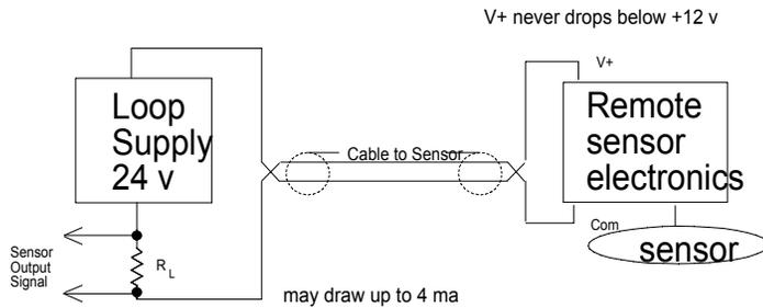
Figure 11. 4 to 20 mA analog current loop
