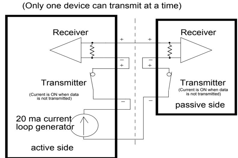
Figure 2. Simplex 20 mA Circuit
